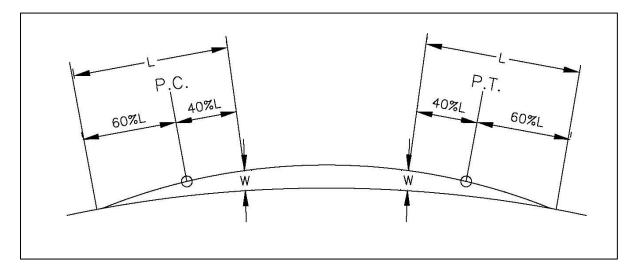
Figure 3-12 Widening on a Simple Curve
