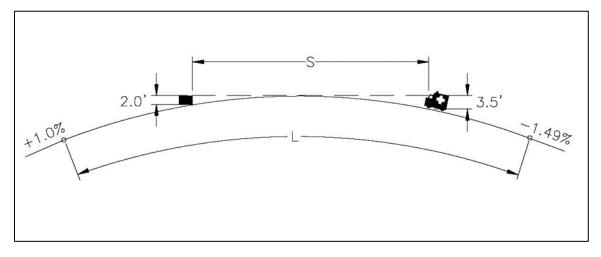
Figure 3-6 Example of Crest Vertical Curve
