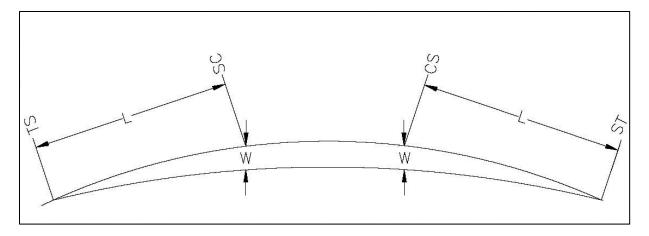
Figure 3-13 Widening on a Spiral Curve
