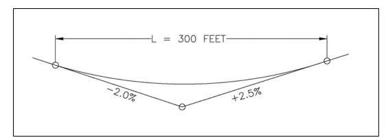
**Figure 3-7 Example of Sag Vertical Curve**
