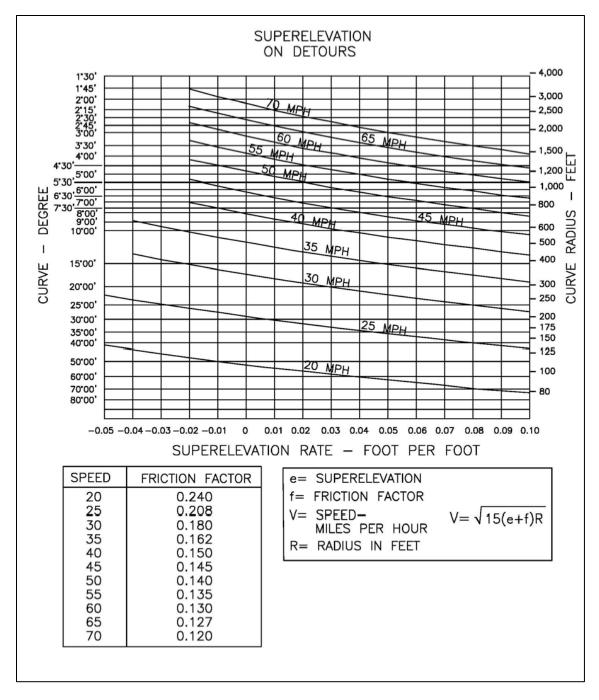
**Figure 3-16 Superelevation on Detours**
